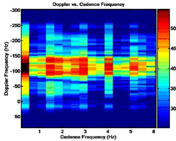
**Figure 5.** Cadence frequency plot for a human target (2 sec. of data).
