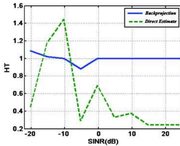
Figure 8. Comparison of backprojection and direct estimates against SINR, for a true HT value of 1 m.
