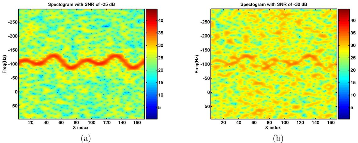
**Figure 6.** Spectrogram in noise. (a) SINR = -25 dB. (b) SINR = -30 dB.
