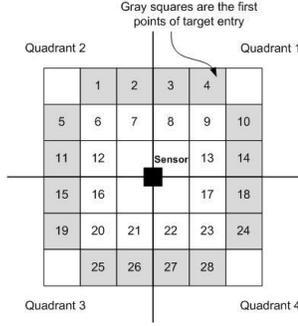
Figure 3. Sensor sensing region discretization.
