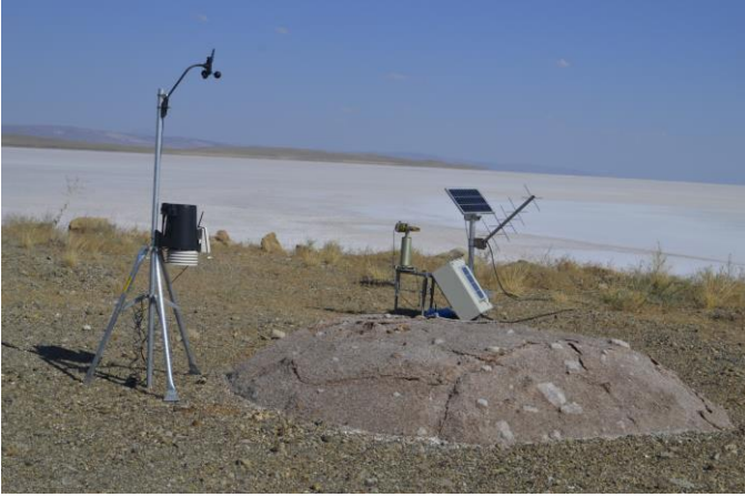
Figure 6 Meteorological Station Vantage Pro 2Plus (left) and Cimel CE318-2 Sun-photometer (right) at Salt Lake
