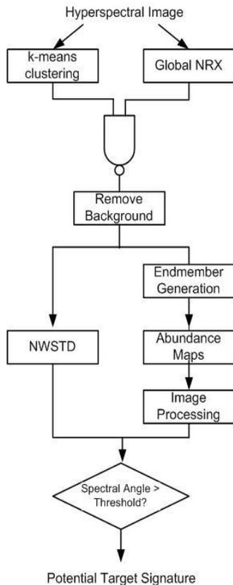
Figure 1. Flow chart for SSE signature extraction algorithm.
